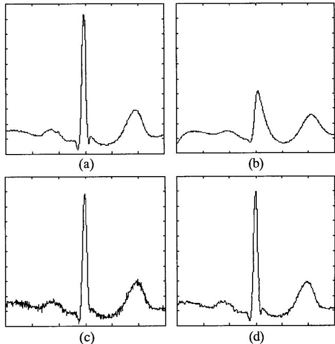
Fig. 3. (a) Original ECG signal,  $f$ , (b) observed signal,  $a_0$ , by ambulatory ECG system ( $L=2$ ), (c) restored signal ( $M=2$ ), and (d) restored signal ( $M=4$ ).
