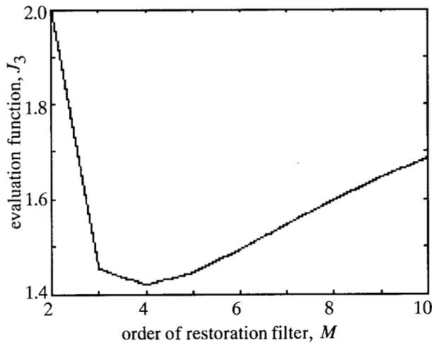
Fig. 2. Optimum order of the restoration filter. ( $L=2$ ,  $s_1, s_2=0.03 \pm j0.04$ ,  $s_0=0.005$ ,  $\sigma=10^{-8}$ ).
